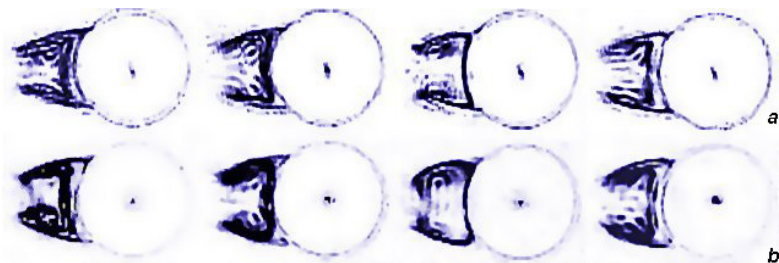
Fig. 4. Examples of two orthogonal views (a and b) of shape and wake of 0.8 mm diameter bubbles (dark-field circular filters in the schlieren cutoff planes).
